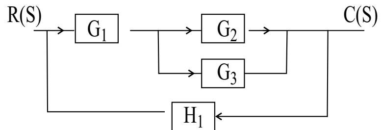
Q.19 Draw basic block diagram of closed loop basic Control System.
